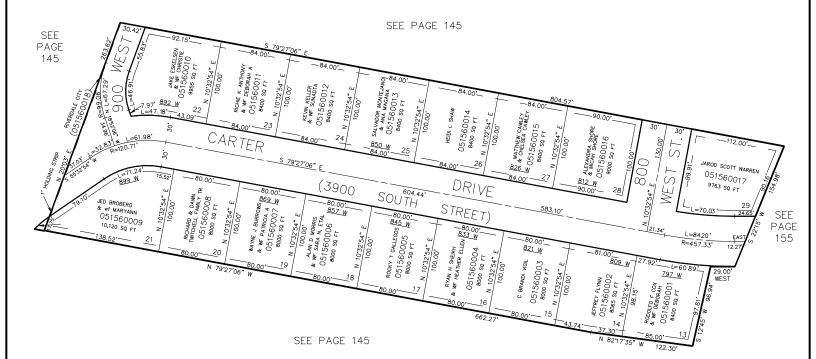
7' UTILITY & DRAINAGE EASEMENTS EACH SIDE OF PROPERTY LINES AS INDICATED BY DASHED LINES EXCEPT AS OTHERWISE SHOWN.
