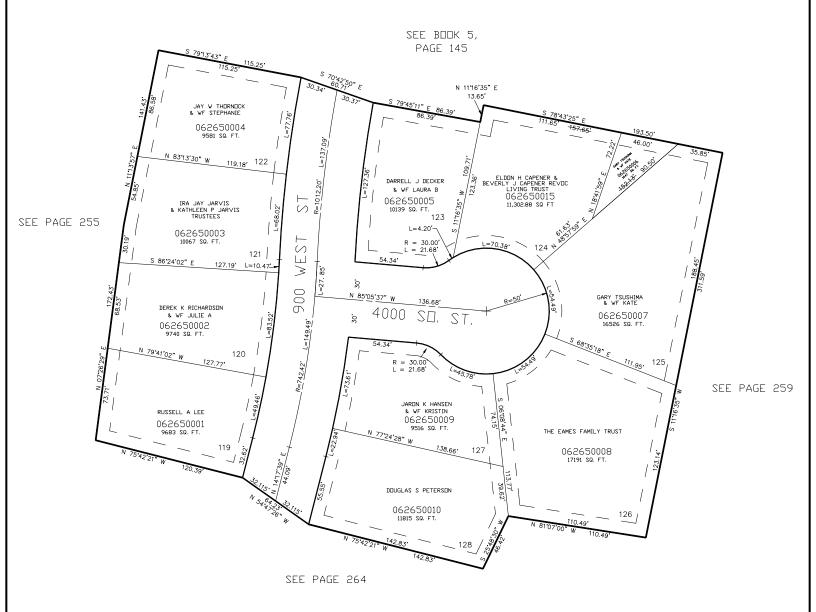
10' UTILITY & DRAINAGE EASEMENTS EACH SIDE DF PROPERTY LINES AS INDICATED BY DASHED LINES EXCEPT AS OTHERWISE SHOWN.
