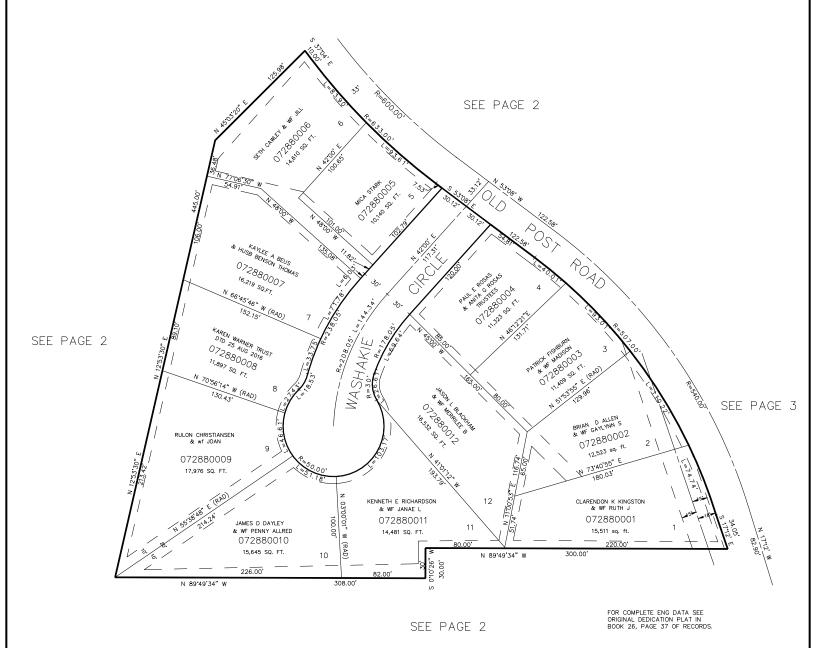
7' UTILITY AND DRAINAGE EASEMENTS EACH SIDE OF PROPERTY LINE AS INDICATED BY DASHED LINES, EXCEPT AS OTHERWISE SHOWN.
