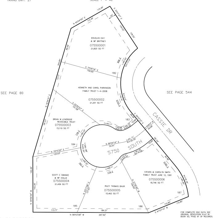
10' UTILITY & DRAINAGE EASEMENTS EACH SIDE DF PROPERTY LINES AS INDICATED BY DASHED LINES EXCEPT AS OTHERWISE SHOWN.
