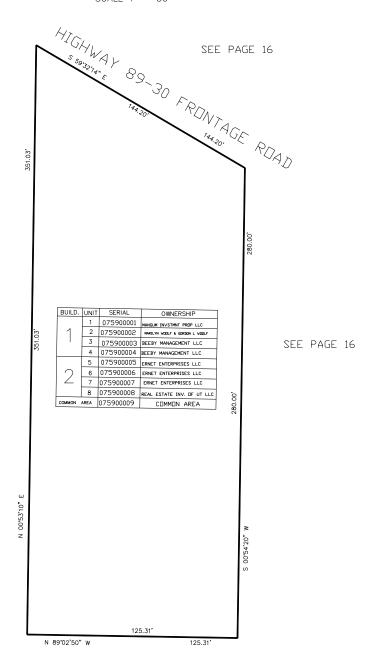
10' UTILITY & DRAINAGE EASEMENTS EACH SIDE DF PROPERTY LINES AS INDICATED BY DASHED LINES EXCEPT AS OTHERWISE SHOWN.
