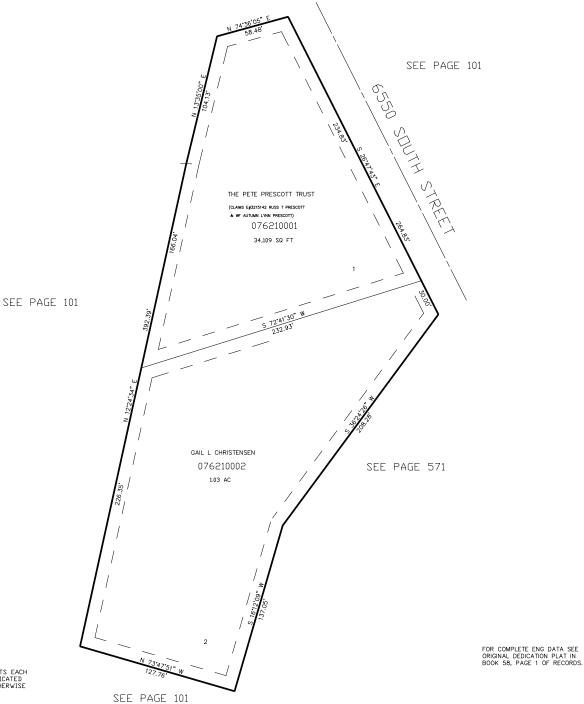
10' UTILITY & DRAINAGE EASEMENTS EACH SIDE OF PROPERTY LINES AS INDICATED BY DASHED LINES EXCEPT AS OTHERWISE SHOWN.
