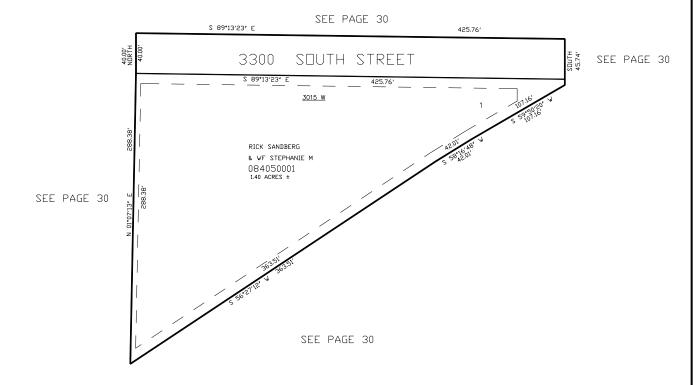
10' UTILITY & DRAINAGE EASEMENTS EACH SIDE OF PROPERTY LINES AS INDICATED BY DASHED LINES EXCEPT AS OTHERWISE SHOWN.
