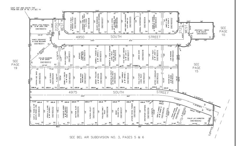
5' UTILITY & DRAINAGE EASEMENTS EACH SIDE OF PROPERTY LINES AS INDICATED BY DASHED LINES EXCEPT AS OTHERWISE SHOWN.
