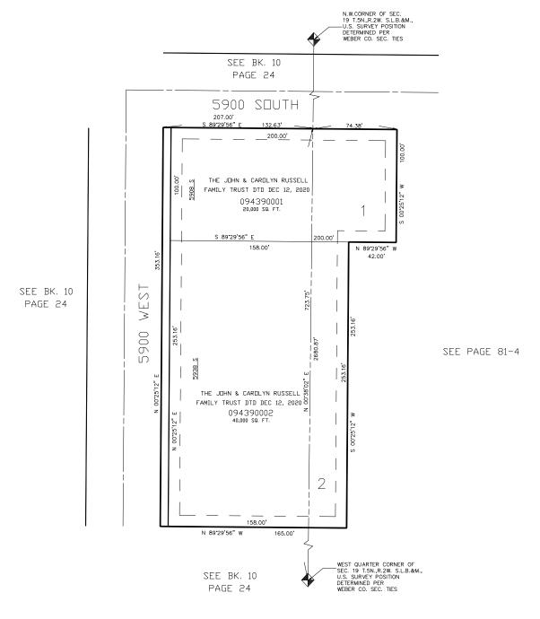
10' UTILITY & DRAINAGE EASEMENTS EACH SIDE OF PROPERTY LINES AS INDICATED BY DASHED LINES EXCEPT AS OTHERWISE SHOWN.
