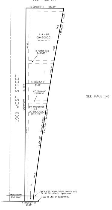
10' UTILITY & DRAINAGE EASEMENTS EACH SIDE OF PROPERTY LINES AS INDICATED BY DASHED LINES EXCEPT AS OTHERWISE SHOWN.
