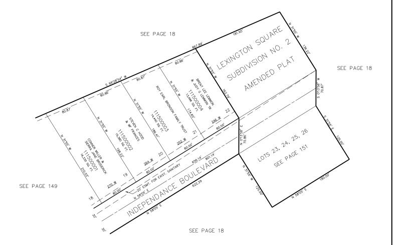
7' UTILITY & DRAINAGE EASEMENTS EACH SIDE OF PROPERTY LINES AS INDICATED BY DASHED LINES EXCEPT AS OTHERWISE SHOWN.
