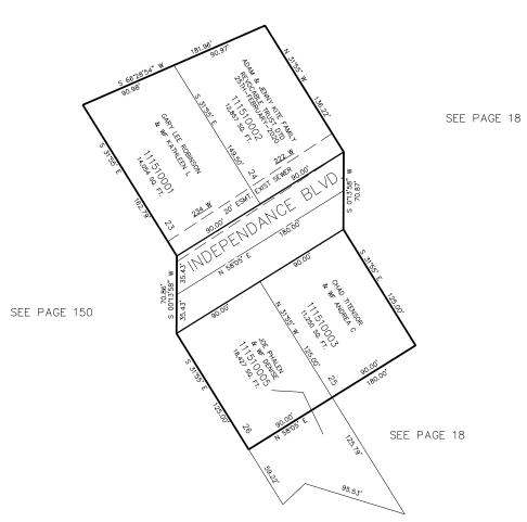
7' UTILITY & DRAINAGE EASEMENTS EACH SIDE OF PROPERTY LINES AS INDICATED BY DASHED LINES EXCEPT AS OTHERWISE SHOWN.
