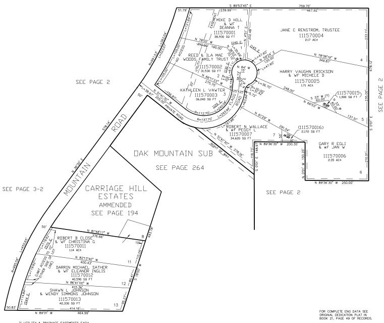
7' UTILITY & DRAINAGE EASEMENTS EACH SIDE DF PROPERTY LINES AS INDICATED BY DASHED LINES EXCEPT AS OTHERWISE SHOWN.
