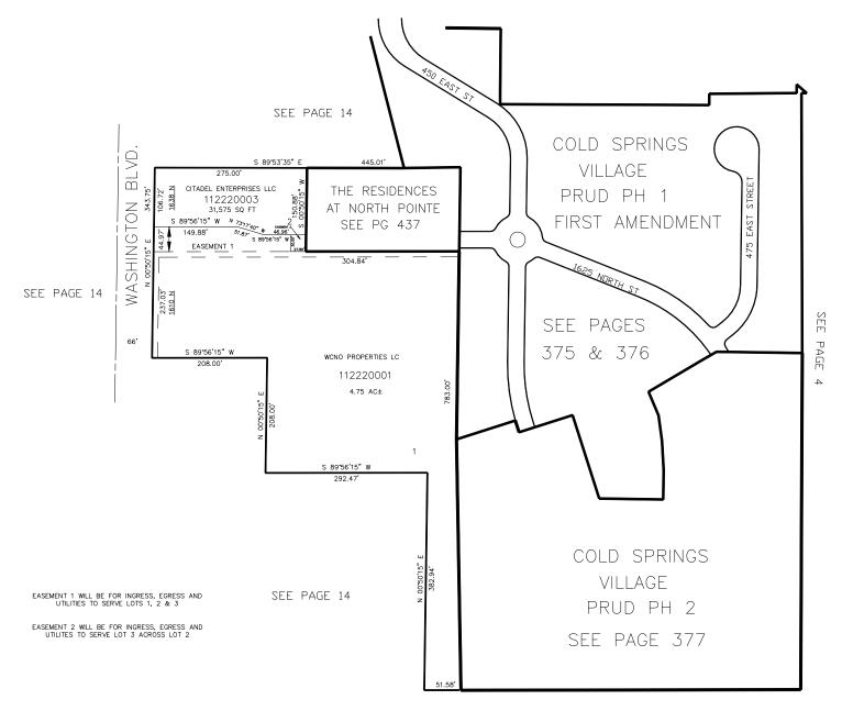
10' UTILITY & DRAINAGE EASEMENTS EACH SIDE DF PROPERTY LINES AS INDICATED BY DASHED LINES EXCEPT AS OTHERWISE SHOWN.
