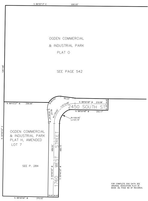
10' UTILITY & DRAINAGE EASEMENTS EACH SIDE OF PROPERTY LINES AS INDICATED BY DASHED LINES EXCEPT AS DTHERWISE SHDWN.
