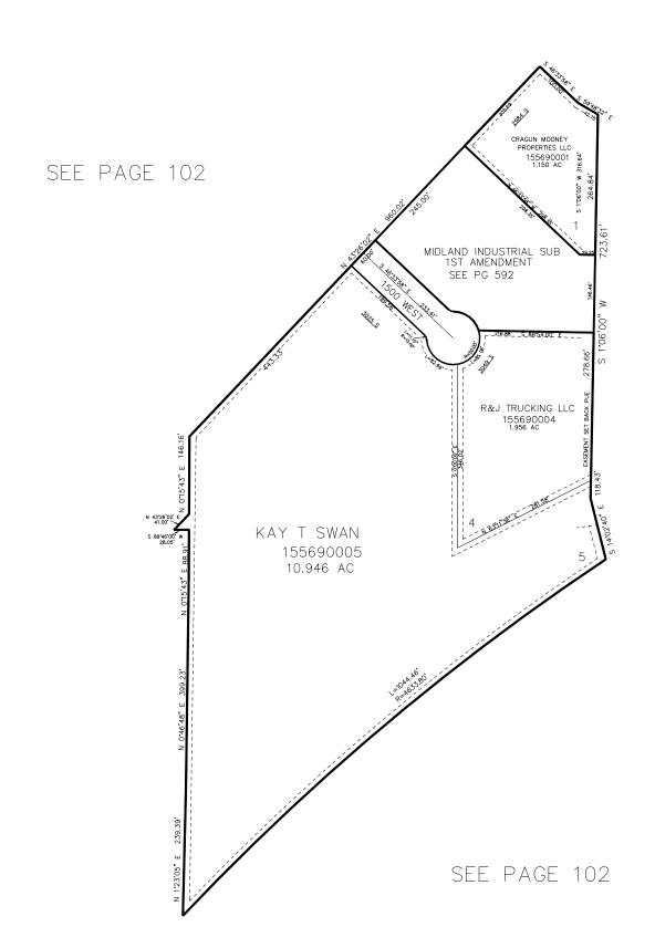
10' UTILITY & DRAINAGE EASEMENTS EACH SIDE OF PROPERTY LINES AS INDICATED BY DASHED LINES EXCEPT AS OTHERWISE SHOWN.
