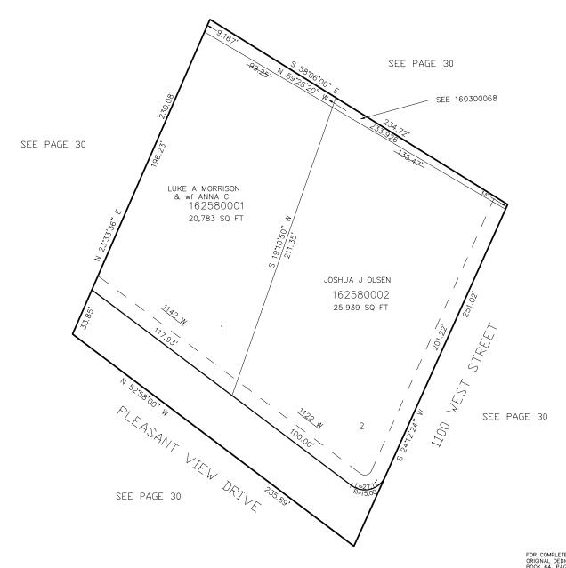
10' UTILITY & DRAINAGE EASEMENTS EACH SIDE OF PROPERTY LINES AS INDICATED BY DASHED LINES EXCEPT AS OTHERWISE SHOWN.
