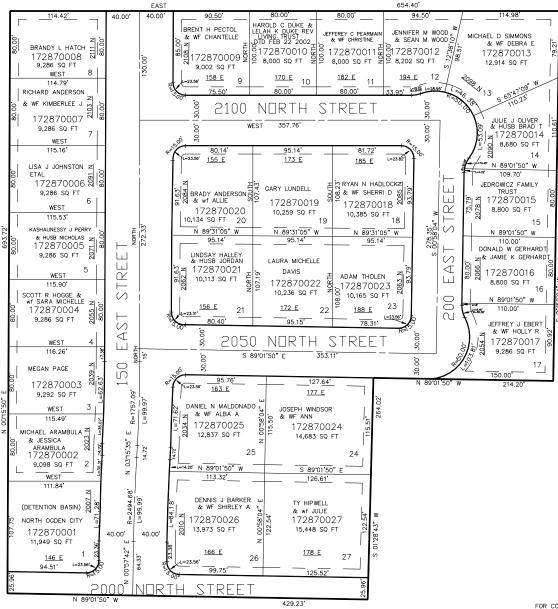
10' UTILITY & DRAINAGE EASEMENTS EACH SIDE OF PROPERTY LINES AS INDICATED BY DASHED LINES EXCEPT AS OTHERWISE SHOWN.
