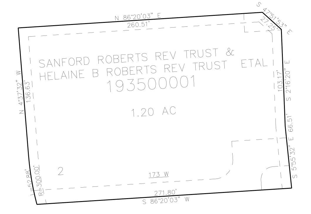
10' UTILITY & DRAINAGE EASEMENTS EACH SIDE OF PROPERTY LINES AS INDICATED BY DASHED LINES EXCEPT AS OTHERWISE SHOWN.
