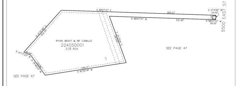
10' UTILITY & DRAINAGE EASEMENTS EACH SIDE OF PROPERTY LINES AS INDICATED BY DASHED LINES EXCEPT AS OTHERWISE SHOWN.
