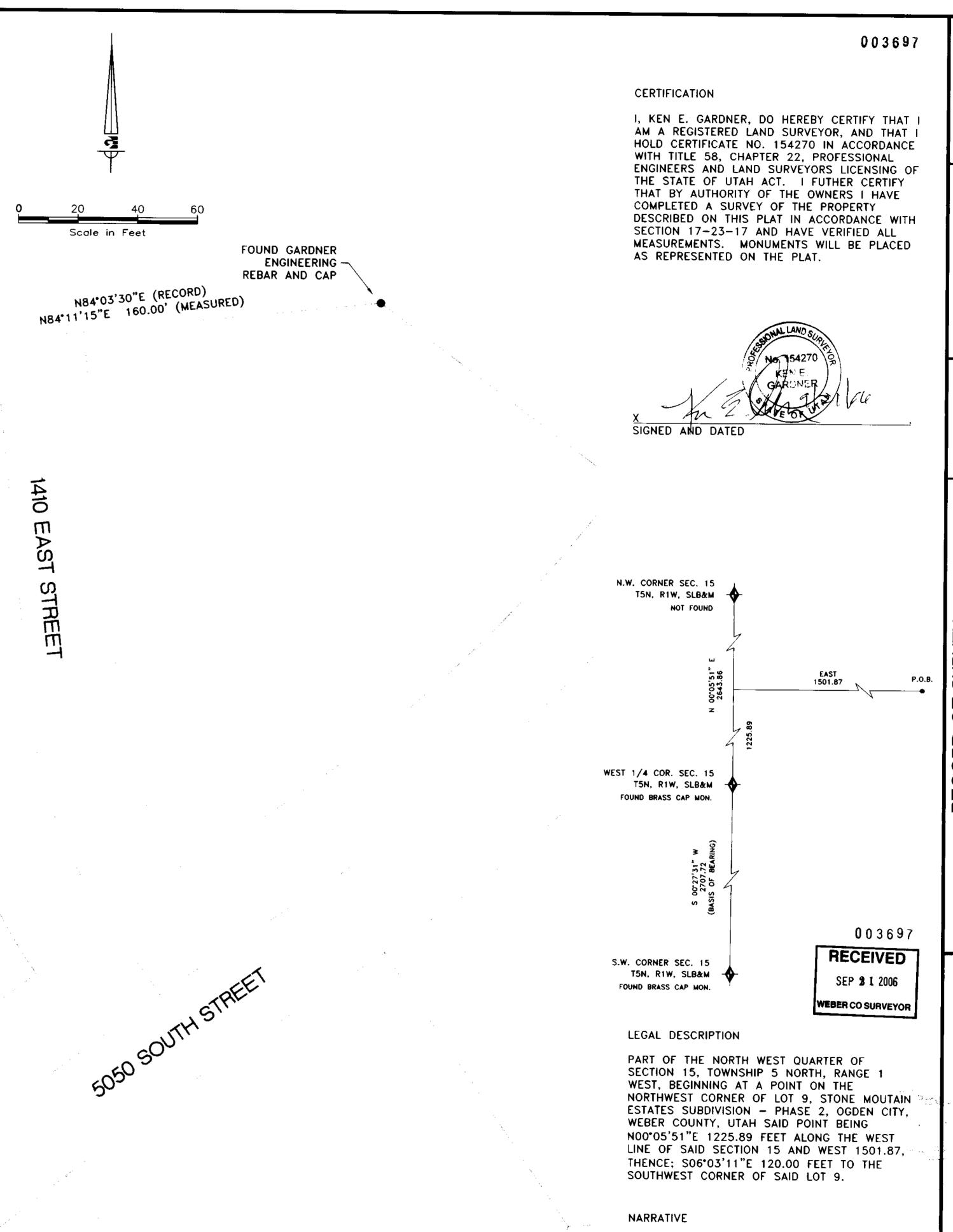
STONE MOUNTAIN TRACT "A" **ESTATES SUBDIVISION** PHASE 4 N05\*56'30"W (RECORD) N05\*48'45"W 42.01 (MEASURED) FOUND GARDNER - ENGINEERING REBAR AND CAP N84°03'30"E (RECORD) N84°11'15"E 116.57' (MEASURED) S06\*10'56"E (RECORD) FOUND REBAR S06'03'11"E 5.13' (MEASURED) AND CAP (UNREADABLE) S83°49'04"W (RECORD) S83°56'49"W 140.00' (MEASURED) − P.O.B. STONE MOUNTAIN ESTATES SUBDIVISION PHASE 2 LOT 9 LOT 7
