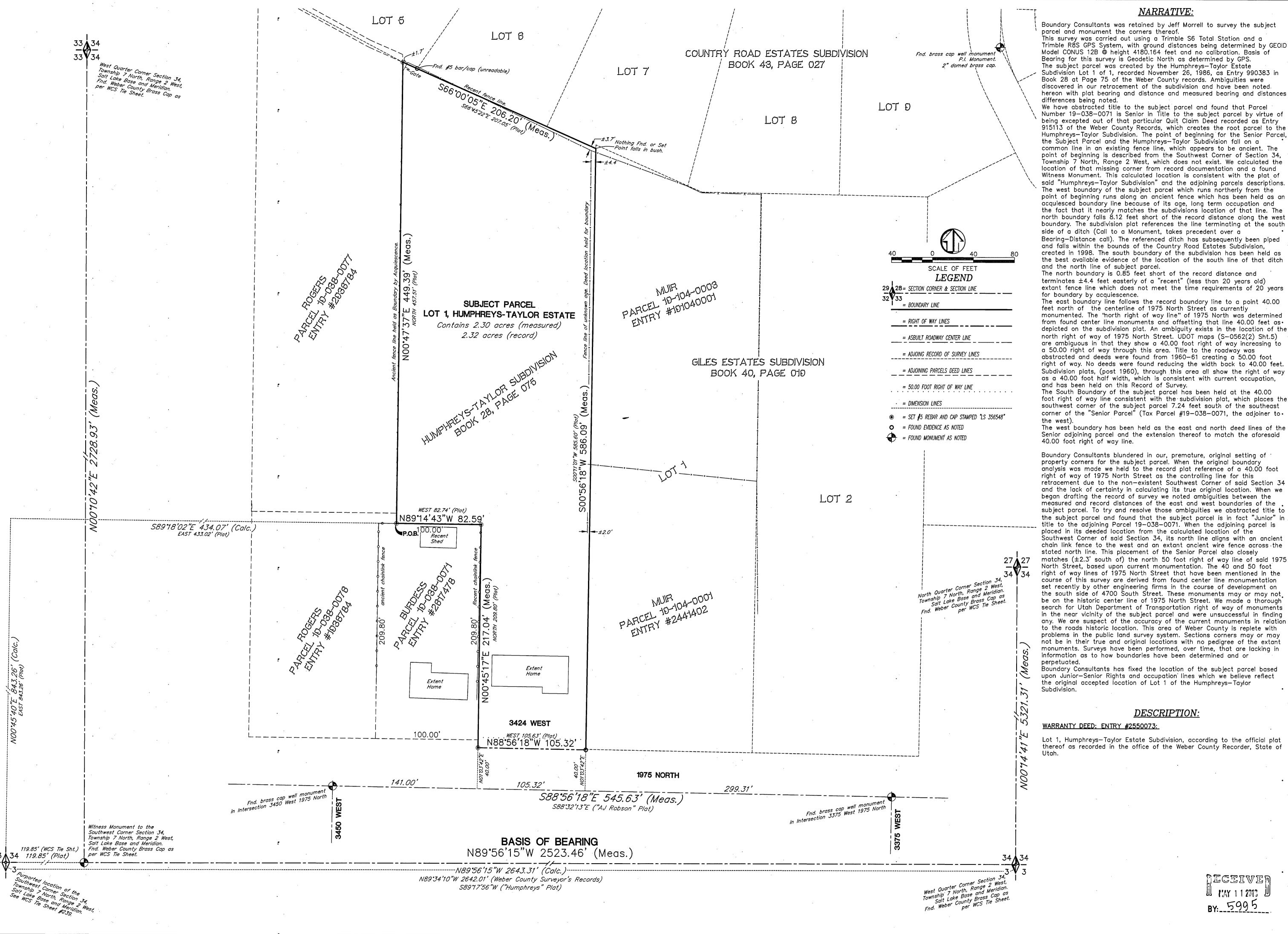
This survey was carried out using a Trimble S6 Total Station and a Trimble R8S GPS System, with ground distances being determined by GEOID Model CONUS 12B @ height 4180.164 feet and no calibration. Basis of
