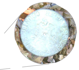
Southwest 16th Quarter Corner to Section 36 T8N, R1W SLB&M (Found Brass Cap)
