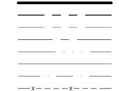
CENTERLINE DITCH TOP BANK FIELD SEPARATION LINE FENCE LINE FOUND REBAR SET BY OTHERS SET 5/8"X24" REBAR WITH CAP SECTION CORNER
